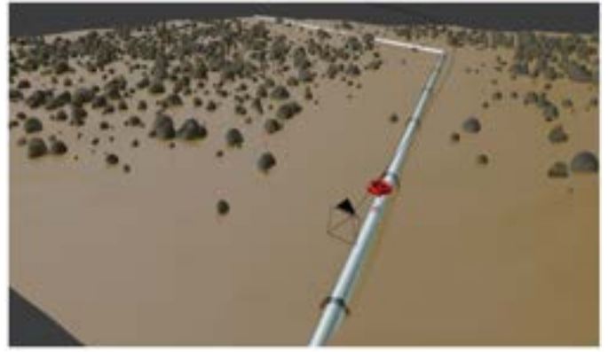
Fig. 5. Example of a randomized Blender scene with seafloor, pipeline, boulders, and sensor trajectory.
